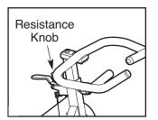
To stop the flywheel, push the brake lever downward. The flywheel should quickly come to a complete stop.
