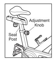
knob is engaged in an adjustment hole in the seat post.
