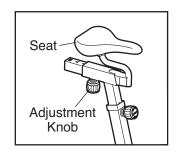
Make sure that the adjustment knob is engaged in an adjustment hole in the seat carriage.
